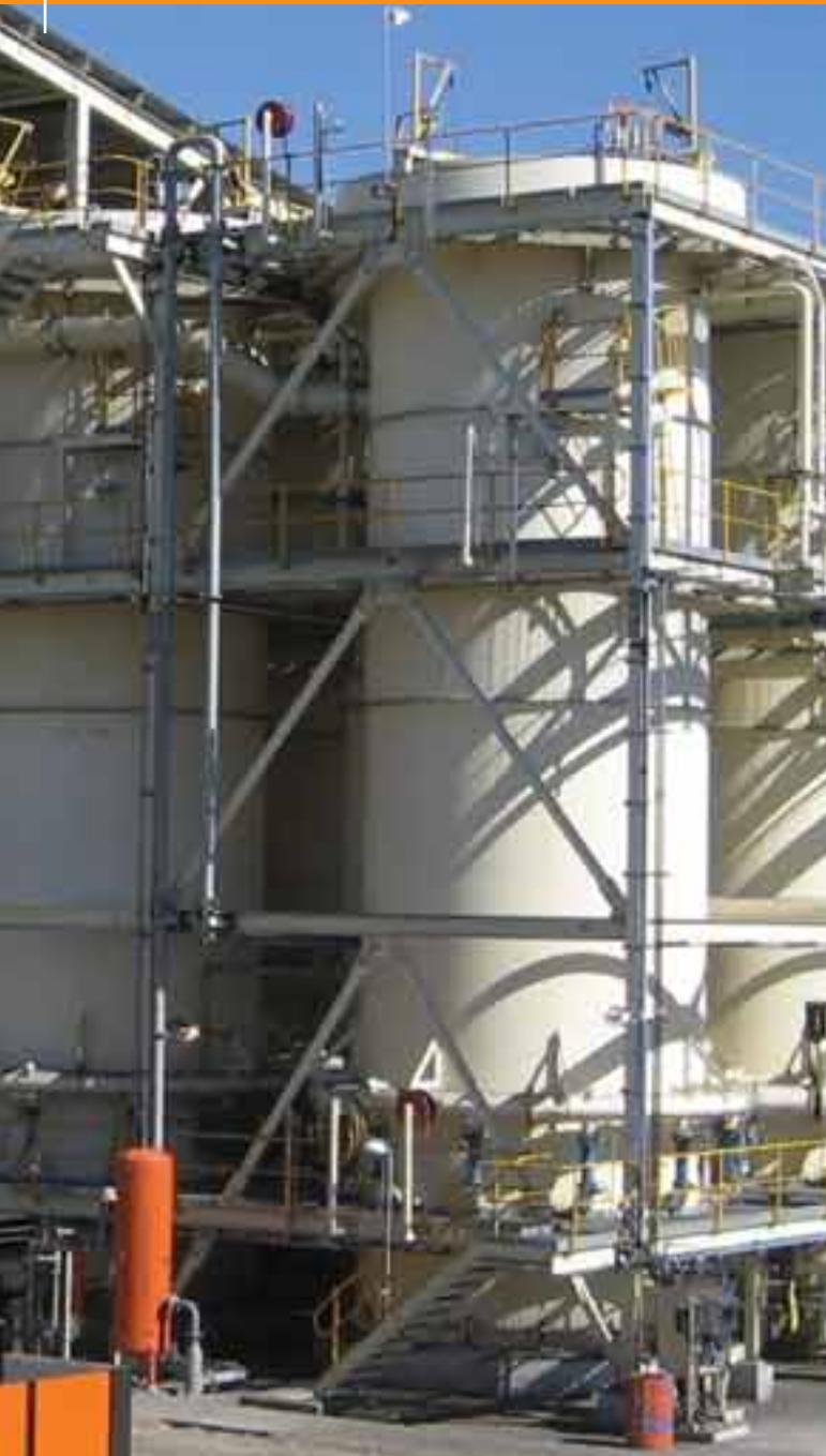
*These Microcel units are used for cleaning freshly mined coal at large mines in Australia.*
